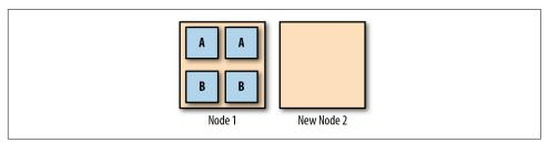
Figure 5-2. After the failure of Node 2, all replicas have moved to Node 1
