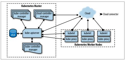
Figure 3-2. How the Kubernetes components fit together
